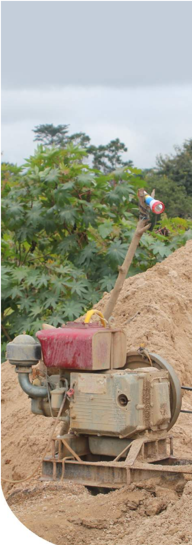
A “Chan fa” machine. A popular hammer mill used by small scale miners, West Africa. Photo: Lynda Lawson
