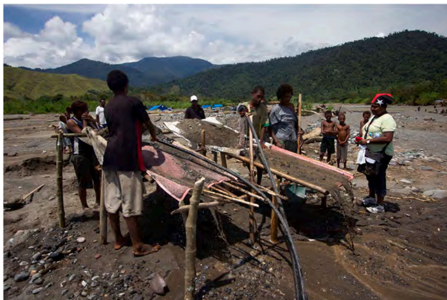
Fig. 6. Small-scale miners using informal equipment to sluice for gold at Madzim village, Wampar Rural LLG, on 17 April 2012. Photo: John Burton.
